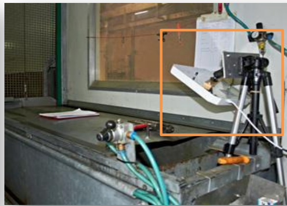
Figure 5.8 - RFID reader at Stun Box
