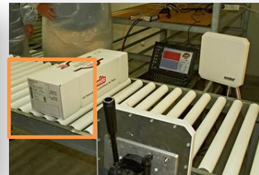
Figure 5.11 – Tagged cartons moving from boning room to chiller room
