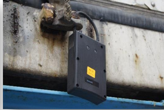
Figure 7.13 – RFID tag secured to the shipping container
