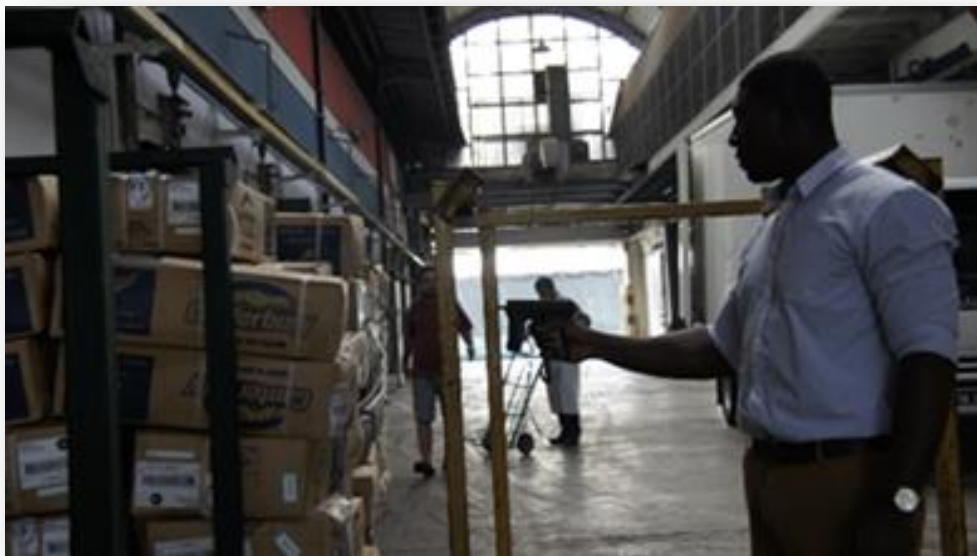
Figure 7.14 - Reading RFID labels on the cartons using a handheld RFID reader
